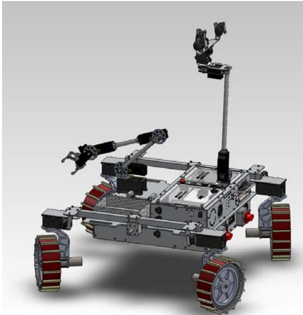
Fig 2. Side View of Rover showing Rocker System
