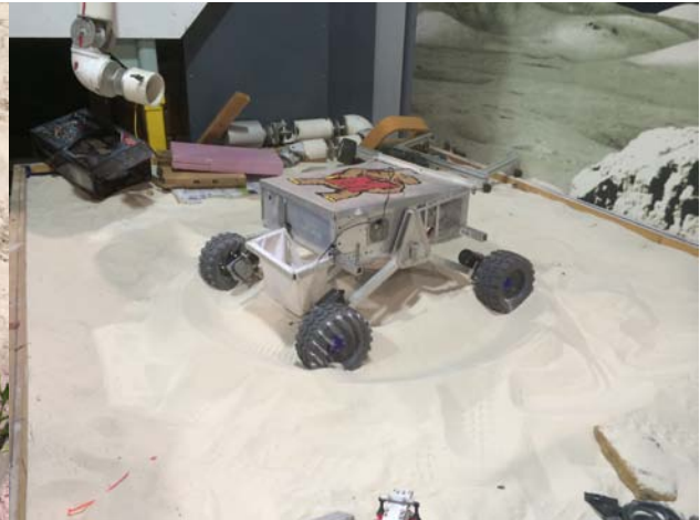
Figure 8: Traction assessment in sand
