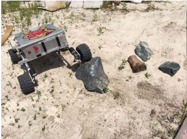
Figure 7: Wheel testing in Moonyard
