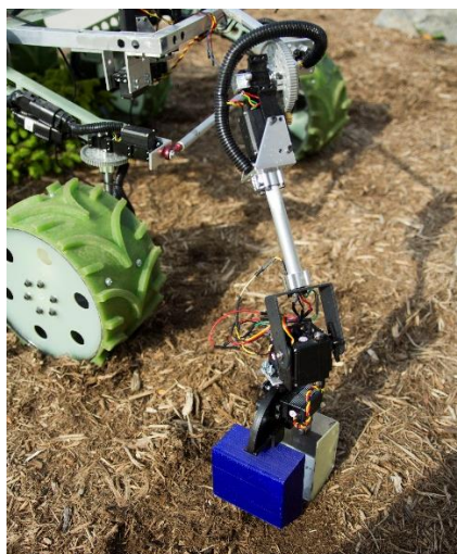
Figure 8 – Rock Manipulating Arm. The system shown above has a total of five degrees of freedom. The five degrees of freedom will allow for a wide range of locations to pick up rocks from and it makes it easier for the operator to do so. Each of the servos has a rotational freedom of 180 degrees.
